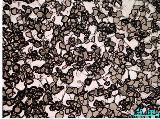
FIG. 1. Microscope image of the ErN crystals grown on the tungsten substrate at 1790 °C. The crystals adopted a predominately (100) orientation due to nucleation on the substrate's grain boundaries. The dark color represents the ErN crystals with average dimensions of 10 \times 5 \times 5 \mu\text{m} .
